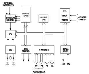
Fig1: Block Diagram of the AT89C core
