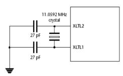
Fig 10: The Microcontroller Clock Input
