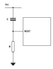
Fig 9: The RC Reset System
