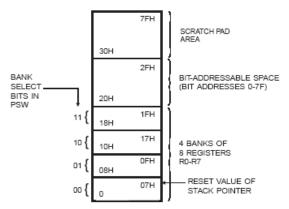
Fig. 6: The Lower 128 Bytes of Internal RAM
