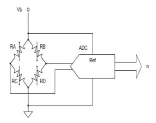
Fig. 8: Ratio-metric Measurement
